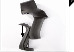
Slide the backstrap off of the pistol grip as seen in Figure 2.
