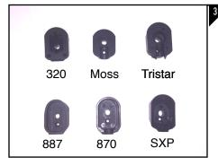
Select the appropriate adapter and screw for your shotgun as seen in Figure 3. NOTE: For the 887 use the 1/4-28 x 1 1/4" screw and # 12 washer and for the 870 use the 1/4-28 x 2" screw and # 12 washer. For the Mossberg use the 5/16-18 x 1" screw and for the SXP, 320 and Tristar use the M8-1.25x50mm Socket Heasd Cap Screw.
