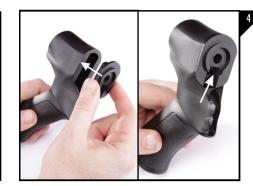
Using the appropriate adapter for your shotgun, place into the pistol grip and using a phillips head screw driver, install and tighten the provided  $6 \times$  $48/2 \times 1/2$ " Plastite Phillips Flat Head screw as seen in Figure 4.
